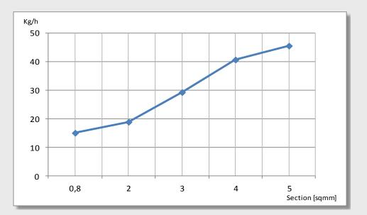
Plant running speeds depend on various factors such as enamel characteristics, copper quality, number of passes and so on. Under normal running conditions, the plant will run the above indicated speed when using good quality materials and enamels by us suggested. The final quality level is in compliance with the IEC standards. During commissioning acceptance test will be considered positive if production speeds values will be reached at 85%
